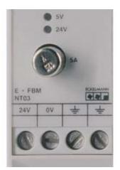
The module electronics are protected by a plug fuse Microfuse 5A, 125V (manufacturer Wickmann, no. 303-1500-042).
