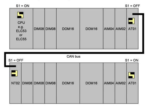
Example for a multi-line system structure of field bus modules
