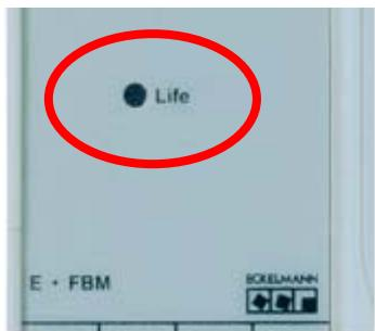
Supply voltage on: As soon as the supply voltage has been switched on, the module is in the state of automatic baud rate recognition. The life LED in the upper part of the module is flashing at 8 Hz. Upon recognition of the baud rate, an internal initialization of the module is made. Subsequently, the module is in the internal state „*Pre-operational*“. The module is now ready for operation and attends control signals via the CAN bus. The life LED is flashing at 0.25 Hz.
