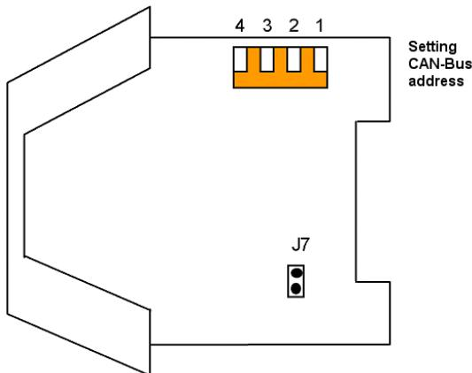
The basis address (higher-value address bits) of the CAN bus can be modified by means of the 4-pole DIL switch. Normally, the preset address should not be modified.
