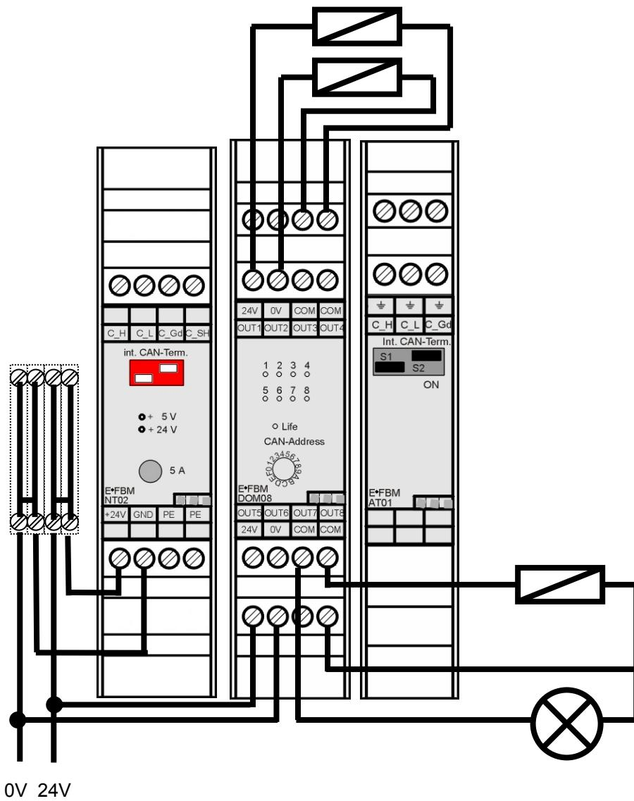
In this example, the 24V supply required for the outputs is externally connected.
