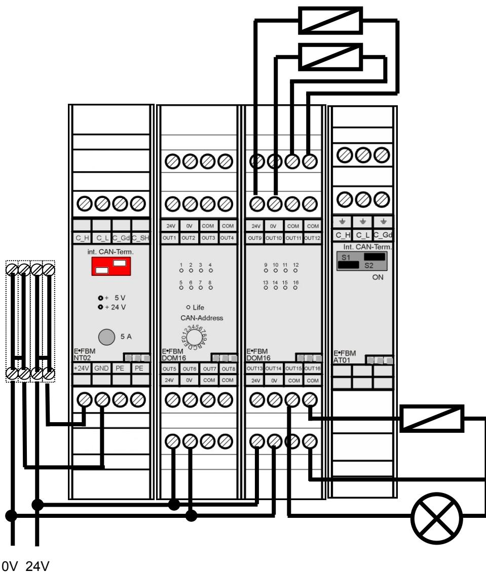
In this example, the 24V supply required for the outputs is externally connected.
