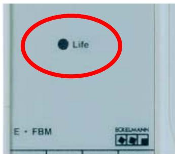
Supply voltage on: As soon as the supply voltage has been switched on, the module is in the state of automatic baud rate recognition. The life LED in the upper part of the module is flashing at 8 Hz. Upon recognition of the baud rate, an internal initialization of the module is made. Subsequently, the module is in the internal state „*Pre-operational*“. The module is now ready for operation and attends control signals via the CAN bus. The life LED is flashing at 0.25 Hz.
