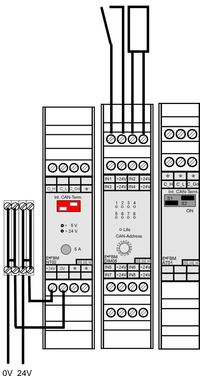
In the example, the 24V supply required for the input signal is taken from the module.
