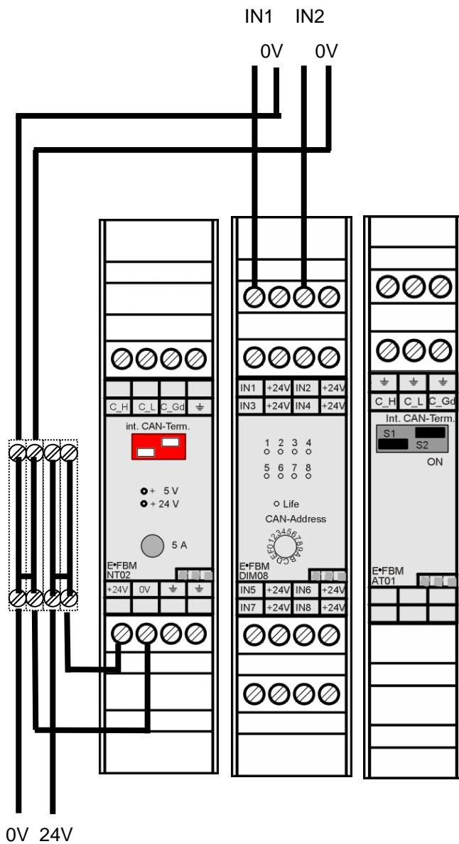
The example shows the connection possibility of an external 24V supply.
