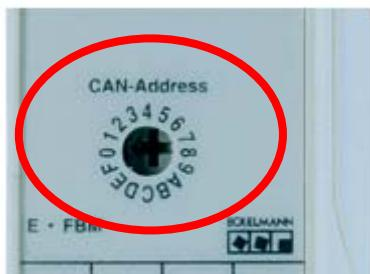
The setting of the node address is made via a hexagonal switch on the front (4 low-value address bits) and via a coding switch inside the housing (3 higher-value address bits). Therefore, max. 16 modules are possible within one module type by coding via the hexagonal switch.
