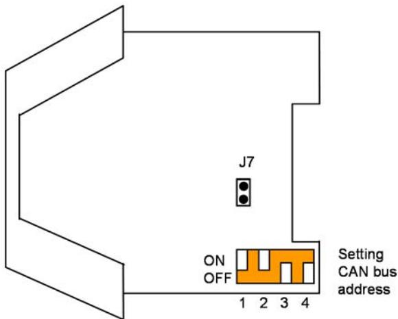
The basis address (higher-value address bits) of the CAN bus can be modified by means of the 4-pole DIL switch. Normally, the preset address should not be modified.
