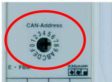
The setting of the node address is made via a hexagonal switch on the front (4 low-value address bits) and via hard-wired bridges inside the housing (3 higher-value address bits). Therefore, max. 16 modules are possible within one module type.
