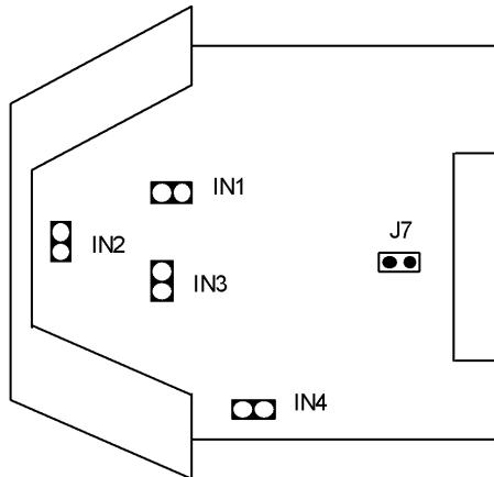
For each input IN1 .. IN4, the respective input can be selected separately as voltage or current input via a bridge.
