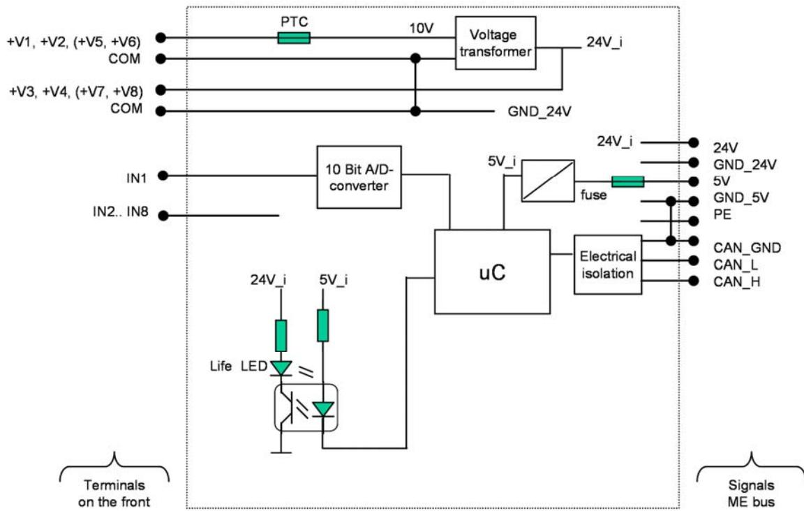
FBMAIM0402: this module has no voltage transformer. Therefore the supply voltage 24V are output at terminal +V1, +V2, +V3, +V4.
