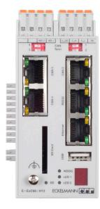
CAN1 CAN2..4 RS232 Ethernet USB WDOG LED1, LED2 SD-Card CAN-Interface with COMBICON connector 3 x CAN-Interface with RI45 Programming interface RS-232 Network connection 10/100 MB USB interface Watchdog LED Status LED CAN1 Slot for SD-cards
