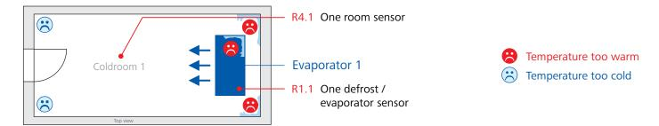
Solution: If required, a bridge circuit composed of 4 sensors of the same type (e.g. L243) located at selected, representative points in the coldroom or evaporator can be used to improve controller behaviour. The bridging circuit can be used for every temperature sensor!
