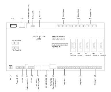
Optional: 2 x CAN-Interface Optional: 1 x EtherCAT<sup>®</sup> 3 serial interfaces Programming interface Ethernet, RS232 Digital inputs and outputs Analog inputs and outputs Analog axis interface for 4 axes PWM interface for laser control
