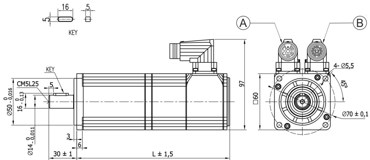
A: Power connection B: Feedback connection
