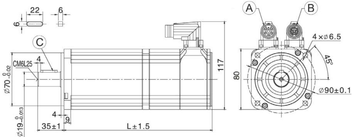
A: Power connection B: Feedback connection C: Key
