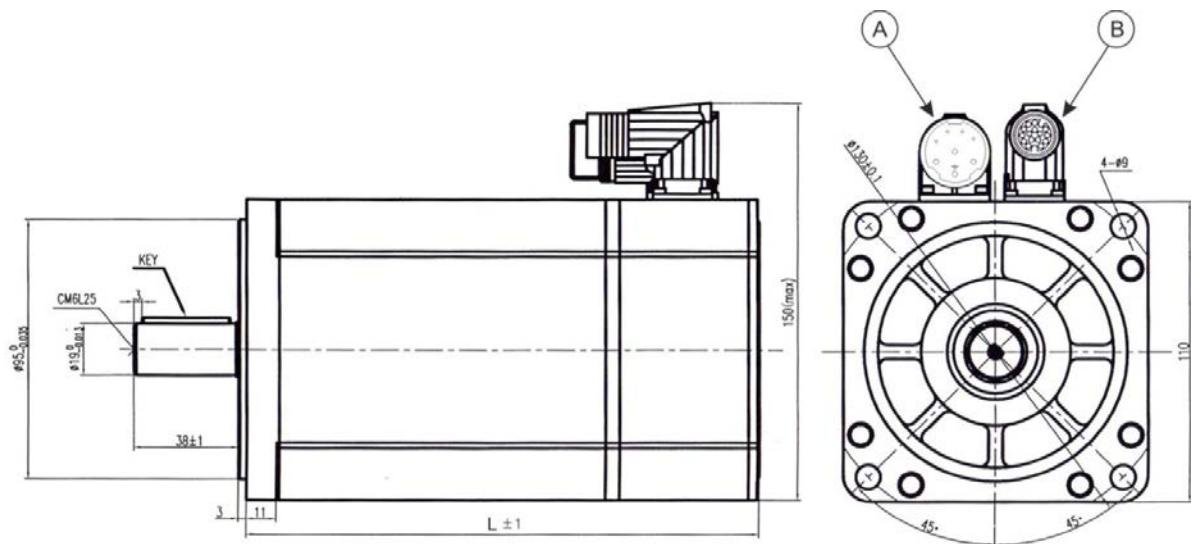
A: Power connection B: Feedback connection
