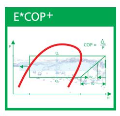
Innovative energy saving functions help enhance the coefficient of performance (COP) of refrigeration systems and heat pumps.
